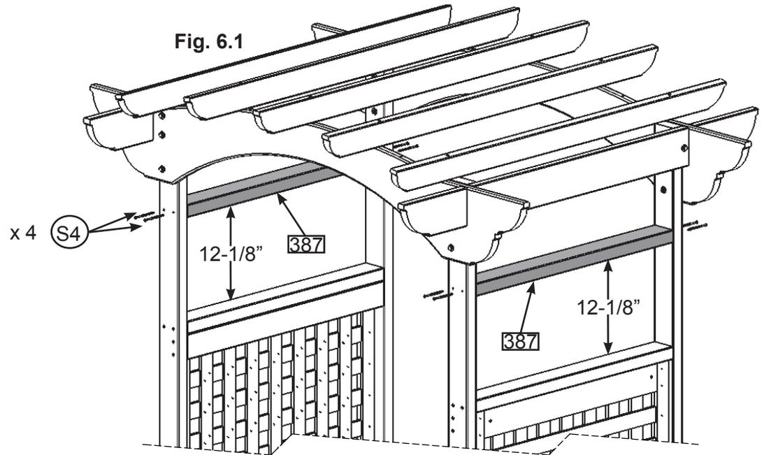
**A:** Attach one (387) per side as shown in fig.6.1 with 4 (S4) Wood Screws.
